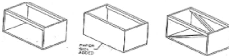
What about putting it all together. Hot glue is great in the speed of assembly department, but you may find that wood glue is stronger and lighter. Screwing the chassis together works well too, but you'll pay a weight penalty there as well. If you do use screws put a little glue on the threads before screwing them in and they will hold better.
