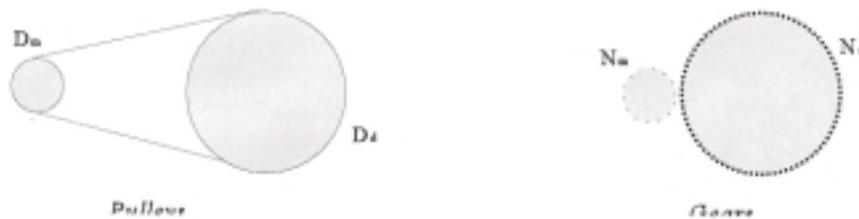
The variable **D** is the diameter of the pulley, variable **N** is the number of teeth on the gear, subscript **d** refers to the gear attached to the drive axle, and subscript **m** is the gear attached to the motor.
