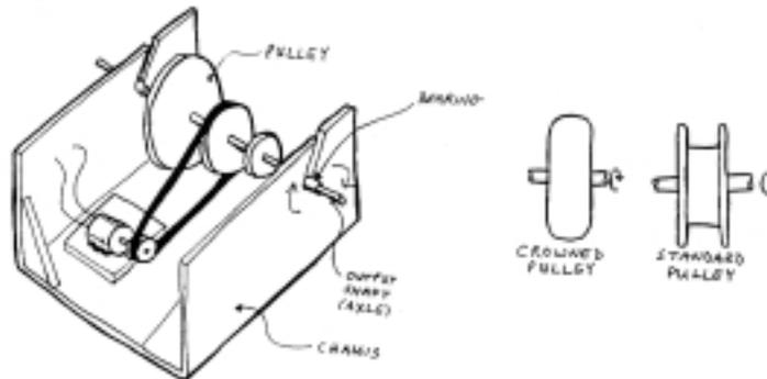
Build a test transmission like the one shown above. Mount the motor on a piece of stiff material (using hot glue, good tape, etc.) that is easy to grip or attach to the chassis. Use it to adjust motor location and belt tension.
