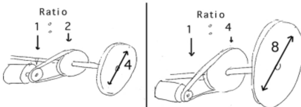
A last note on wheel size, the faster the axle rotates in the bearing the more friction and drag it will have. A larger wheel will allow the axle to rotate more slowly (if the car is to go at the same speed), and will waste less power in the bearings.
